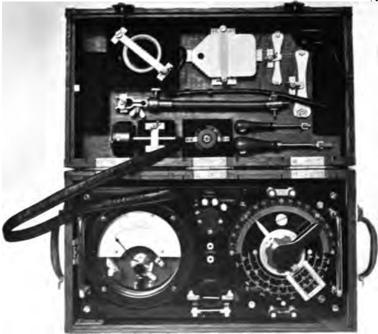
FIG. 91.—Telefunken wavemeter in transport case.
